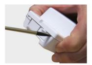
The radiosonde cover can be removed by inserting a flat screwdriver at the two designated spots at the end of the radiosonde.
