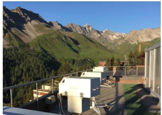
Figure 1 Solar spectrophotometer of the Brewer type on the terrace of the laboratory in Arosa
