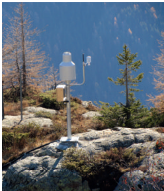
The weather can be measured with automatic observation stations in even the most remote regions in the Alps.
