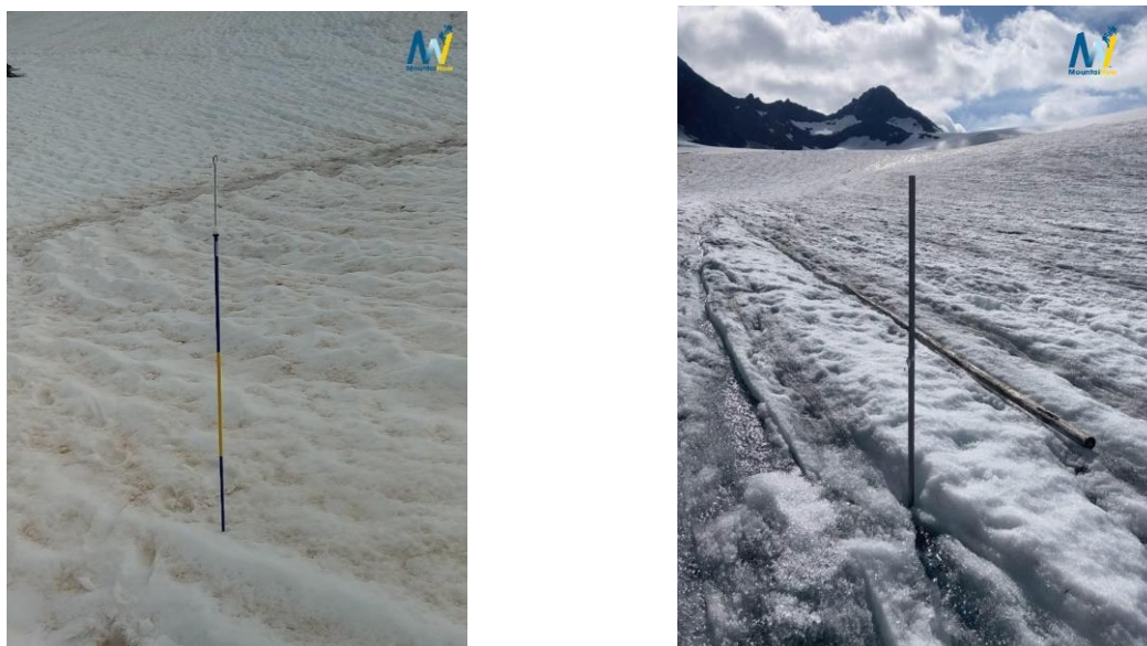
Fig. 5: Observation examples for the (left) “snow depth” variable: snow probe on Glacier du Tsanfleuron; and (right) “glacier melt” variable: ablation stake on Silvrettagletscher
