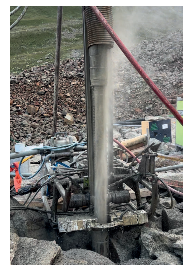
Drilling in rock glacier Muragl (2400 m asl.) in Summer 2024: water coming out of the drill hole where ice was expected. Photo: J. Noetzli.
