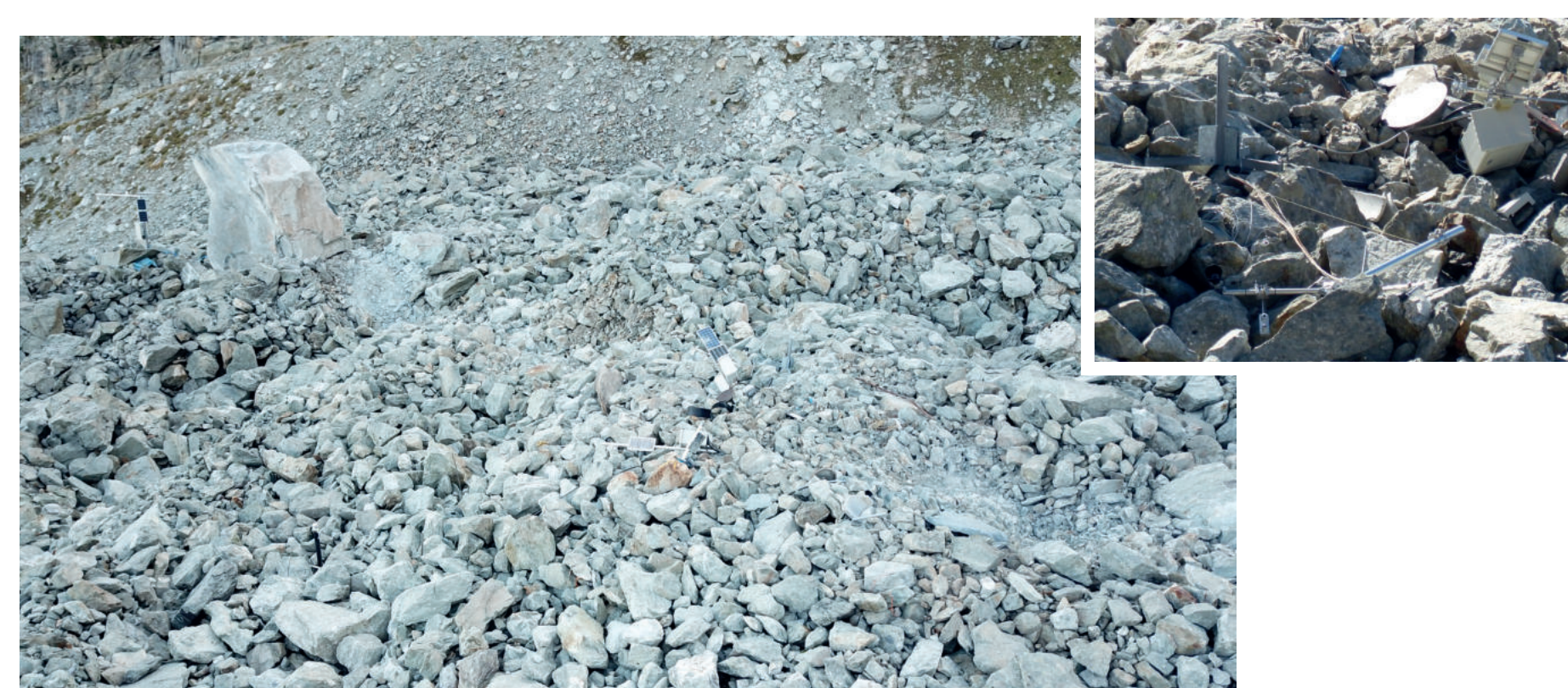
In September 2023, a rock fall hit the field site on rock glacier Murtèl-Corvatsch, severely damaged the instruments, and ended the longest mountain permafrost temperature time series. Photos: Drone Univ. Zurich (left), J. Noetzli (right).
