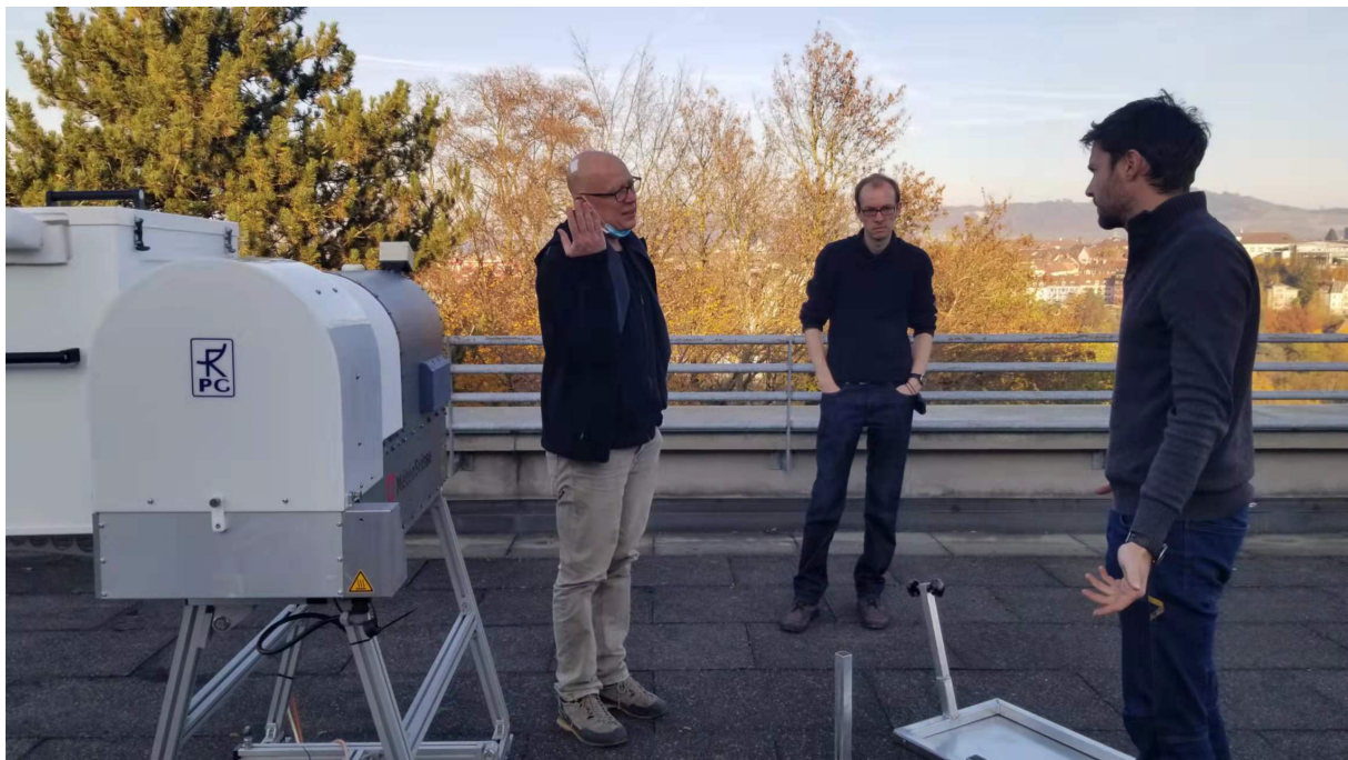
Figure 1. The HATPRO radiometer (left) was safely transferred from MeteoSwiss (Payerne) to the roof of the EXWI building of the University of Bern in November 2021. Axel Murk (IAP), Christoph Dätwyler (IAP) and Maxime Hervo (MeteoSwiss) discuss the calibration and the operation of the HATPRO radiometer at Bern (from left to the right). The water vapour and rain rate measurements of the outdoor HATPRO radiometer can now be compared with the coincident observations of the indoor TROWARA radiometer of IAP.
