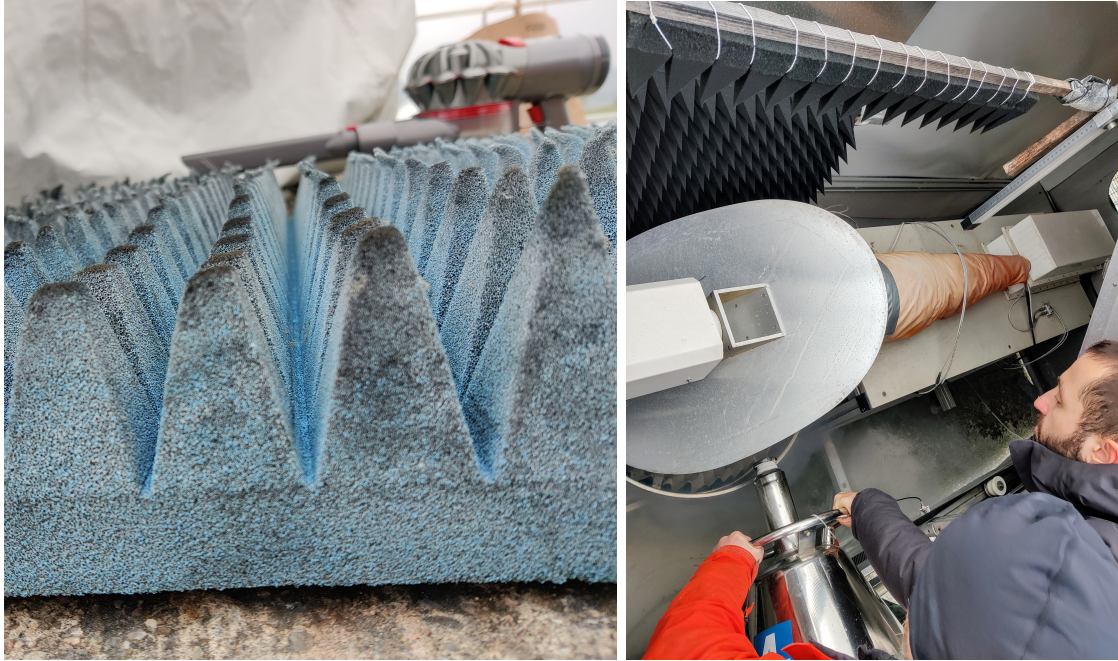
Figure 1: A sideways view of the old ambient target absorber (left) and the instrument during a liquid nitrogen calibration (right). The new reference and ambient absorbers can be seen at the top left of this photo.
