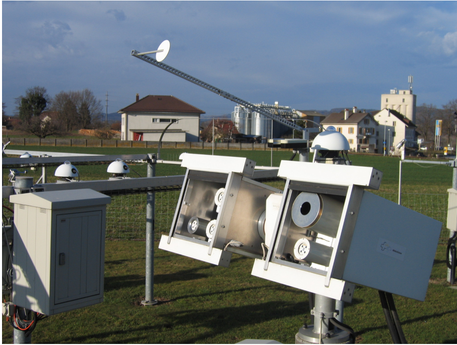
FIG. 2.4: PFR, CH1 NIP and shaded Kipp & Zonen CM21 Pyranometer mounted on a BRUSAG sun tracking instrument
