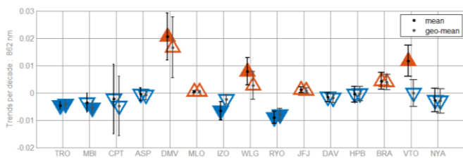
Figure 16b: trends per decade for AOD (mean and geometrical mean) at 862 nm using the WH method
