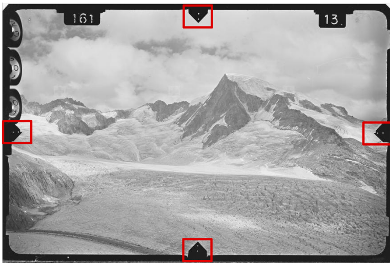
Figure 2: Example of a terrestrial image TerrA (from the type "Wild") acquired over Rhone glacier in 1928. The four fiducial markers have been highlighted in red.
