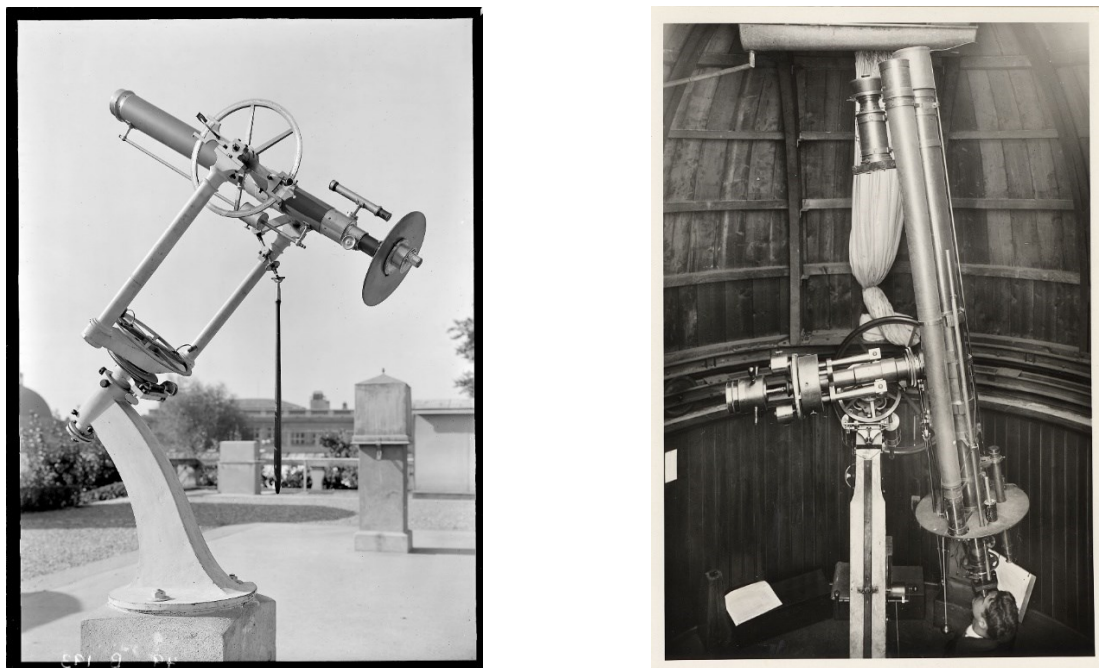
Figure 3 Historical telescopes at the Federal Observatory in Zurich. Left: The Fraunhofer 80 / 1100 mm refractor (64x) on the observation terrace of the Swiss Federal Observatory Zurich - in use since 1855 for daily sunspot observations, photo from 1949. - ETH-Bibliothek Zürich, Bildarchiv: PI_49-B-0193. Right: Solar telescope, ETH Zürich, Eidgenössische Sternwarte, Hauptkuppel, 1930 - ETH-Bibliothek Zürich, Bildarchiv: Ans_05063-003
