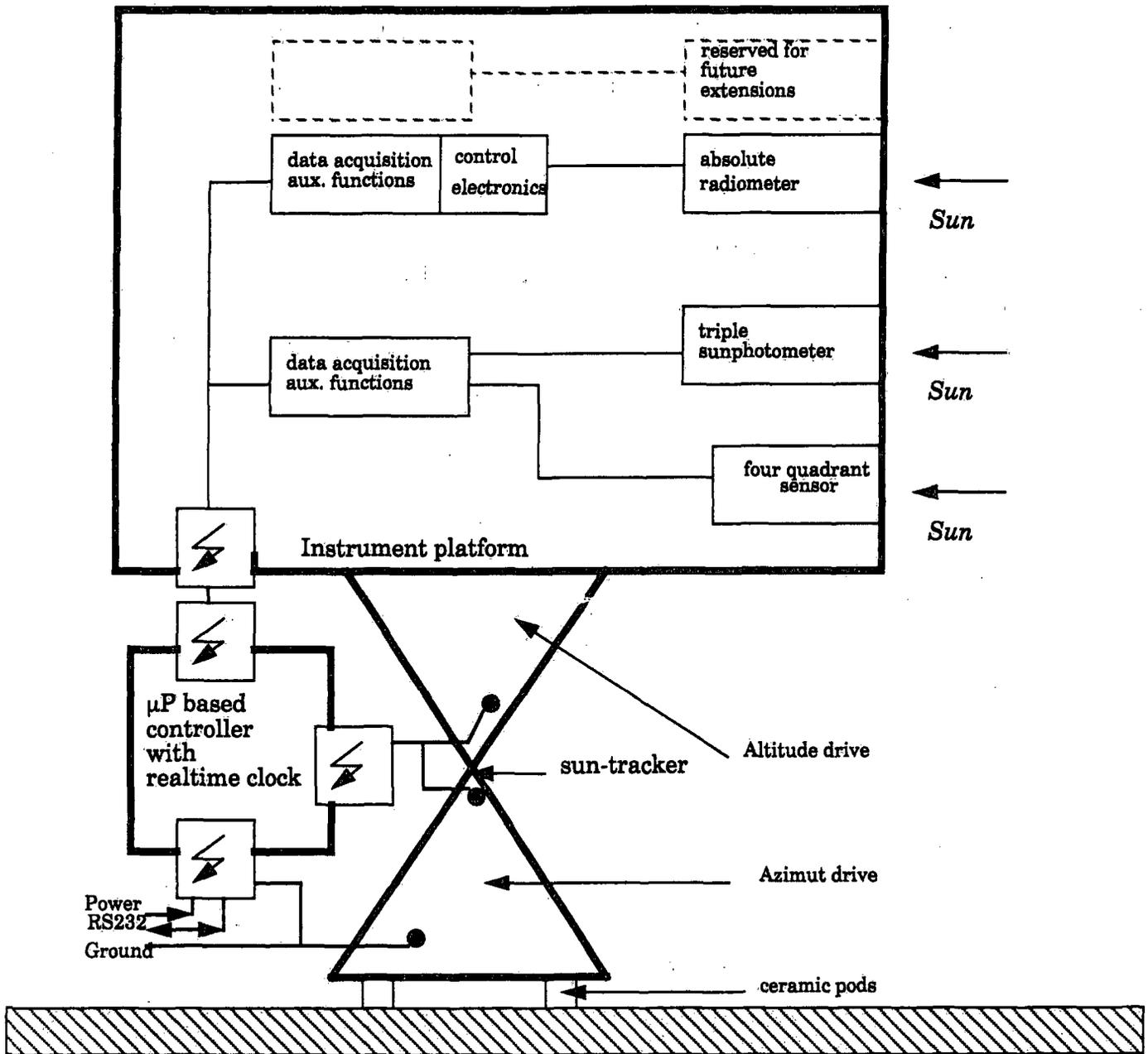
Fig 1: Block diagram of the RASTA units designed for autonomous operation and equipped with an integral lightning protection.
