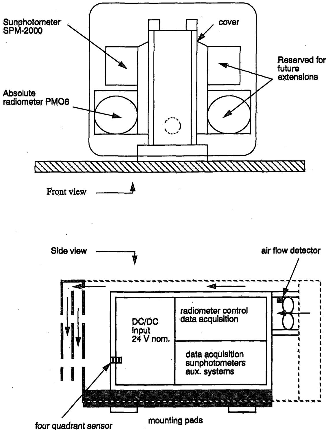
**Fig. 2** Concept of the instrument platform of the RASTA. The precision required prohibits the use of optical windows (rain, dust, etc.). A ventilation system prevents rain, snow, etc. from entering the instrument. The control electronics of the radiometer and the data acquisition electronics are located in the center part of the RASTA housing. The electronics is easily accessible by lifting the left or the right cover. The instruments then move with the cover but keep their line of sight.
