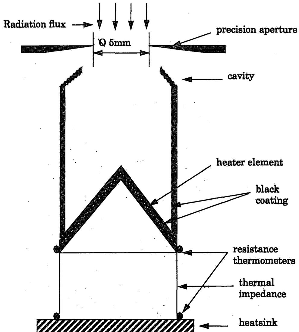
Fig. 3: Schematic drawing of the cavity units of the PMO6-type radiometer
