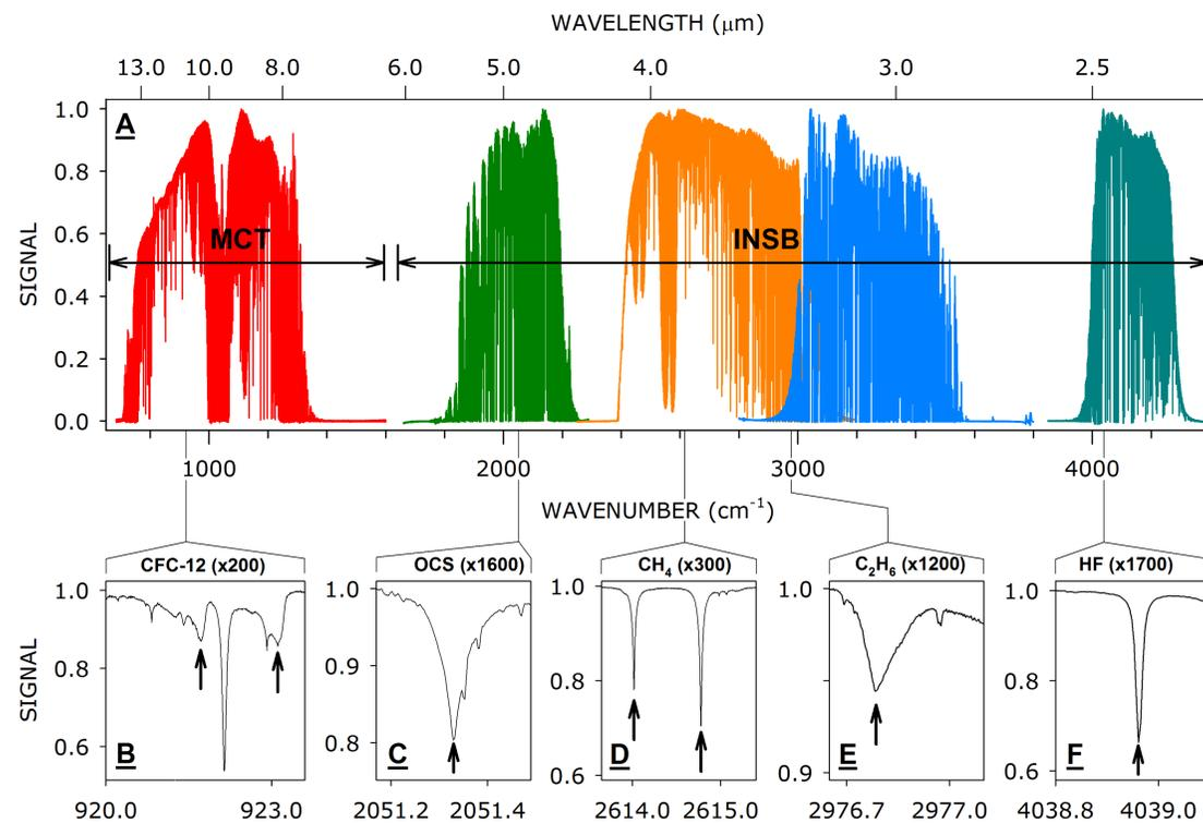
**FIGURE 1.** The spectral ranges routinely recorded at the Jungfrauoch station with our FTIR spectrometer are reproduced in panel A. Panels B to F show, after an horizontal zooming by 200 to 1700 times, a suite of microwindows used to retrieve some of the target species of our atmospheric monitoring program (Mahieu et al., 2017).
